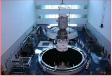
The Shenzhou 9 spacecraft being lifted into the KM-6 thermal vacuum chamber for testing. (credit: Xinhua)
