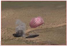
Landing rocket firing and touch-down. Due to strong winds, the capsule did a roll before the parachute was cut. (credit: Xinhua)
