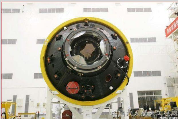
Figure 10 (top): Chinese docking mechanism – active segment. credit: CCTV
