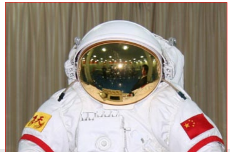
This photo shows the Chinese Feitian EVA suit. It has many similarities with the Russian Orlan-M suit, but there are also many obvious differences between the two suits that may be seen from this front view. (Internet photo)
