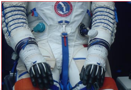
This photo shows exterior details of the Shenzhou IVA suit used by Nie Haisheng in the Shenzhou 6 mission in 2005. (Photo: Chen Lan)
