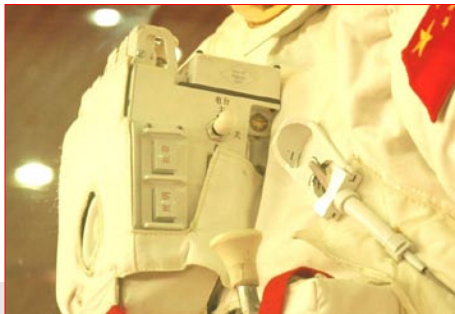
This photo shows equipment mounted at the chest part of the suit. Note the electrical control panel at the far upper part and the gas-liquid controller at the near lower part. (Photo: Jacqueline Myrrhe)
