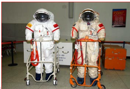
This photo shows the Feitian suit and the Russian Orlan-M suit side-by-side. The Orlan-M suit was used as the backup of the Feitian suit in the Shenzhou 7 mission. In this mission, taikonaut Zhai Zhigang made a 16-minute spacewalk, while Liu Boming only partially emerged from the spacecraft, wearing the Orlan-M suit. (Internet photo)
