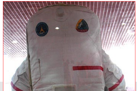
This photo shows the backpack of the Feitian suit. Similar to the Russian Orlan-M, the Feitian suit is a one-piece EVA suit with hatch at back. The backpack is on the hatch cover. (Photo: Jacqueline Myrrhe)
