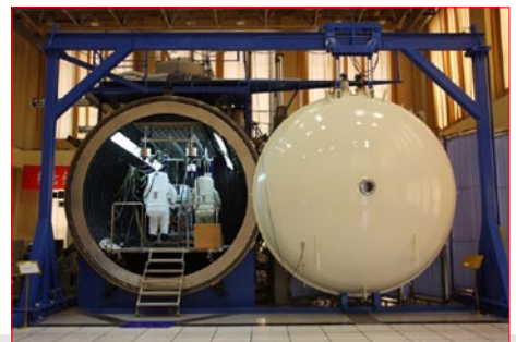
This photo shows the Feitian suit and the Russian Orlan-M suit in a low-pressure chamber test in early 2008. The Orlan-M suit was used as the backup of the Feitian suit in the Shenzhou 7 mission. In this mission, taikonaut Zhai Zhigang made a 16-minute space walk, while Liu Boming only partially emerged from the spacecraft wearing the Orlan-M suit. (Internet photo)
