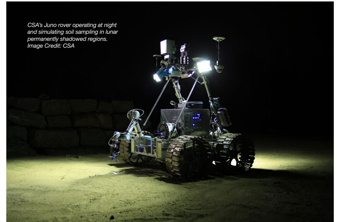
CSA's Juno rover operating at night and simulating soil sampling in lunar permanently shadowed regions. Image Credit: CSA
