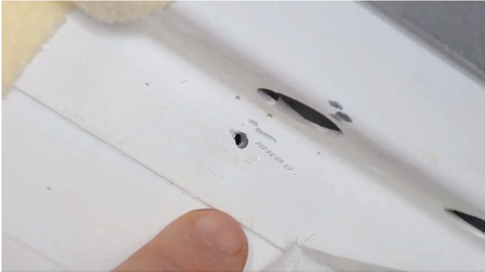
Fig. 10.8. Hole inside the orbital compartment of Soyuz MS-09. Marks show where the drill slipped. (NASA)
