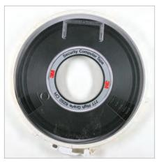
Astronomers once stored telescope data on 9-track tapes. Credit: Hannes Grobe, Wikimedia, CC BY-SA 2.5 (bit.ly/ccbysa2-5)
