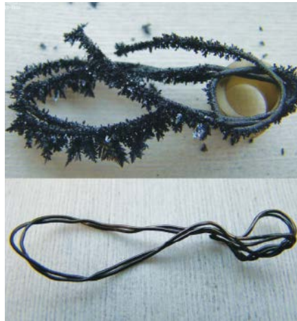
Some types of metal wiring react at Venus-like surface conditions, causing electronics to break down. Shown here is a metal wire before (top) and after (bottom) a test in the GEER chamber. Credit: GEER/NASA Glenn Research Center
