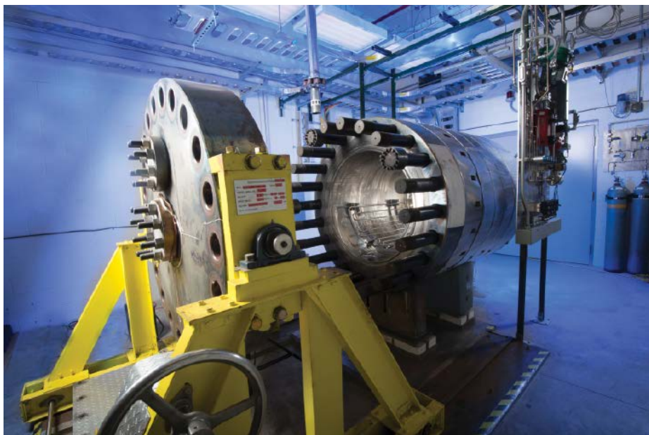
The inside of the Glenn Extreme Environments Rig (GEER) is 1 cubic meter in volume, or about 3 feet wide × 4 feet long. Credit: GEER/NASA Glenn Research Center
