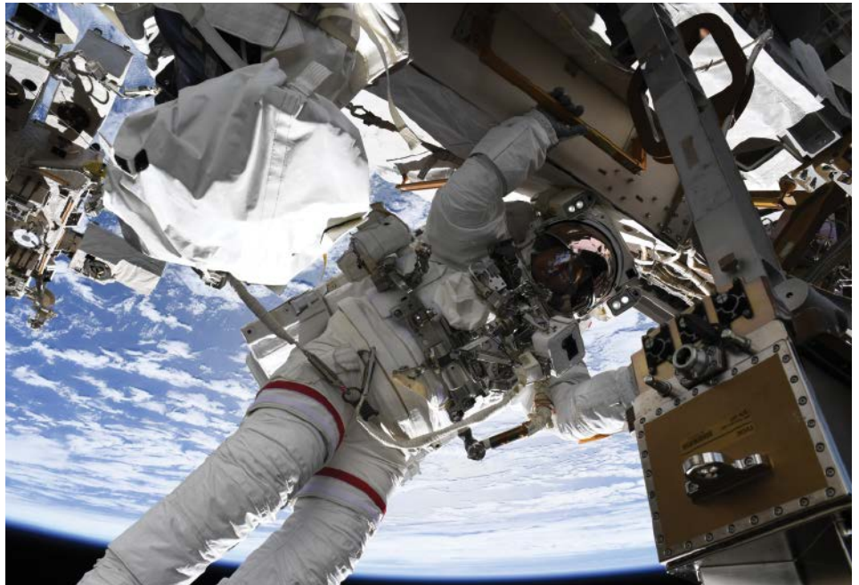
During a 16 May space walk, Drew Feustel installs external wireless antennas and replaces an external light and camera on the International Space Station's truss. Credit: Ricky Arnold/NASA
