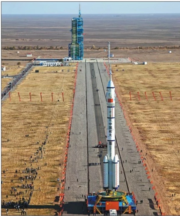
The Shenzhou XIX crew spacecraft and its carrier, a Long March 2F rocket, are moved to the service tower at Jiuquan Satellite Launch Center on Tuesday. LI DONG / FOR CHINA DAILY
