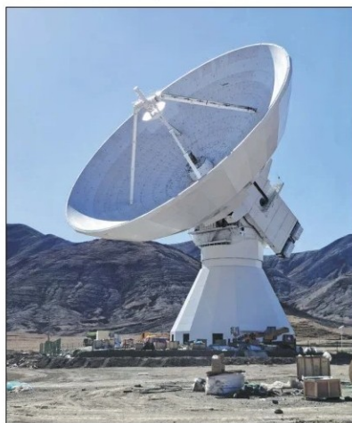
A 40-meter-diameter radio telescope is put into use on Friday in Shigatse, Xizang autonomous region. Built by the Shanghai Astronomical Observatory under the Chinese Academy of Sciences, the telescope aims to offer technical support for the country's lunar and deep-space probe missions. PROVIDED TO CHINA DAILY
