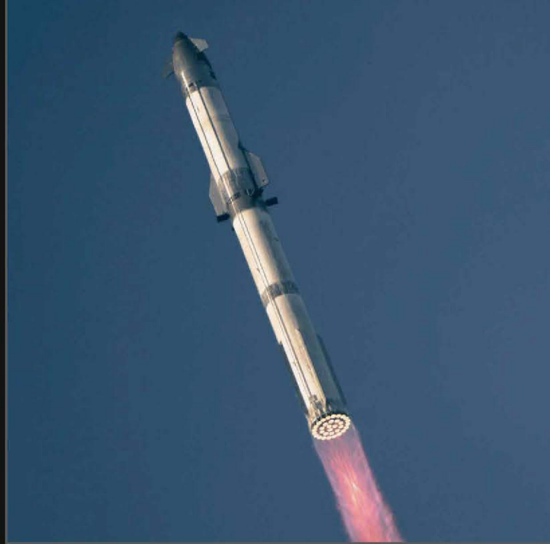
▲ The 16 January launch was the seventh Starship test flight and the first for a slightly taller Block 2 version of the upper stage
