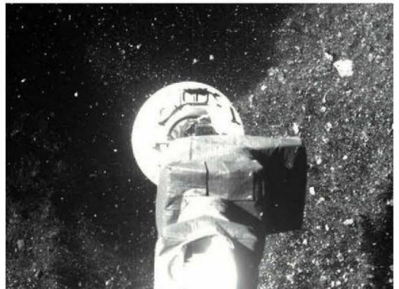
▲ Hit the rocks: OSIRIS-REx's robotic arm snatches its sample in just six seconds of contact in October 2020
