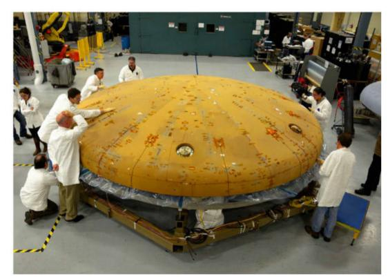
Scientists inspect the Orion spacecraft's heat shield, which has been developed to protect a future crewed mission
