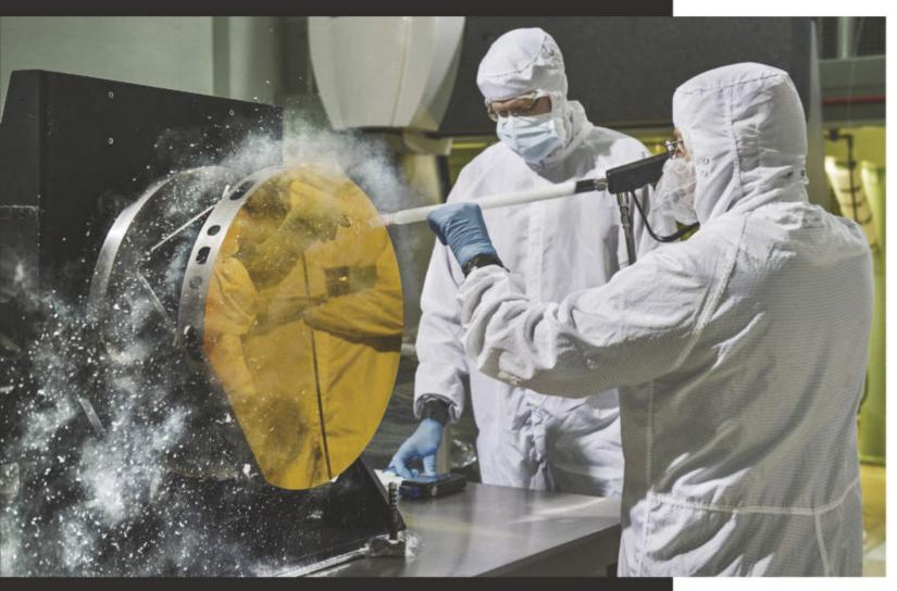
LEFT Small dust particles can greatly affect the science the JWST is able to do, so pristine mirrors are critical. Here engineers practise using carbon dioxide snow to clean a test mirror segment and remove contaminate particulates without scratching the surface.
