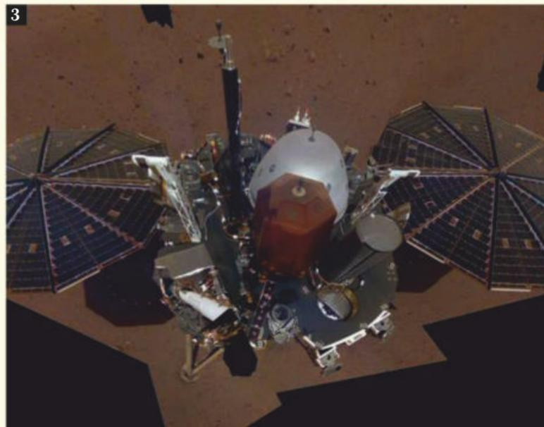
**1.** The polyhedron structure houses SEIS – the seismometer that measures the internal activity of Mars. The dome was placed over SEIS to protect it from the Martian elements.
