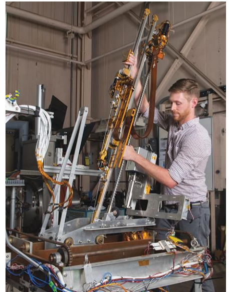
Once scheduled to prospect for lunar ice aboard the VIPER lunar rover, the Honeybee Robotics TRIDENT ice drill will now only operate from the fixed landing site of the Intuitive Machines IM-2 mission. HONEYBEE ROBOTICS
