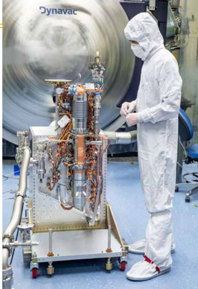
SwRI recently completed assembly and testing of the Mass Spectrometer for Planetary Exploration (MASPEX) to be carried by the Europa Clipper mission. It will search for organic material in Europa's oceans. SWRI
