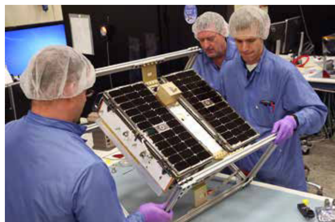
The Cyclone Global Navigation Satellite System (CYGNSS) is assembled and tested at SwRI's satellite facility. The CYGNSS spacecraft underwent thermal vacuum, acoustical, and vibration testing at SwRI prior to launch. SWRI
