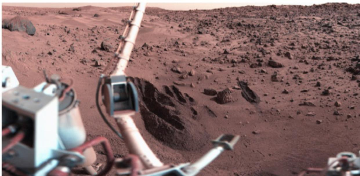
**THE VIKING 1 LANDER** made the first attempts to find life on Mars. The craft's robotic arm dug these trenches and delivered samples to three biology experiments, though the results proved ambiguous at best. NASA/JPL
