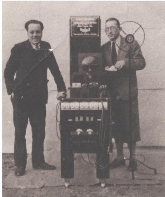
**Figure 1–6:** Otto Paul Fuchs (right) with the sound recorder Photophon. Austrian patent No. 132981/1932, which was acquired by Klangfilm G.m.b.H. Berlin, a subsidiary of Siemens-Berlin.
