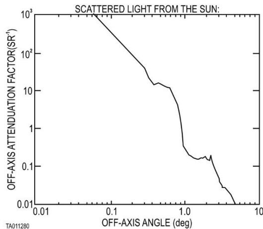
**Figure 7–5:** Voyager Narrow Angle Camera Scattered Light Performance.
