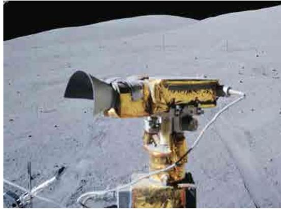
**Figure 22–20:** The RCA camera in the front of the LRV [2].
