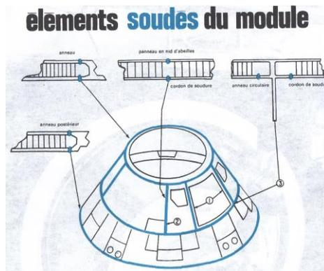
**Figure 22–30 (right):** CM welded elements [Sciaky at Work Vol. 8 no. 10].
