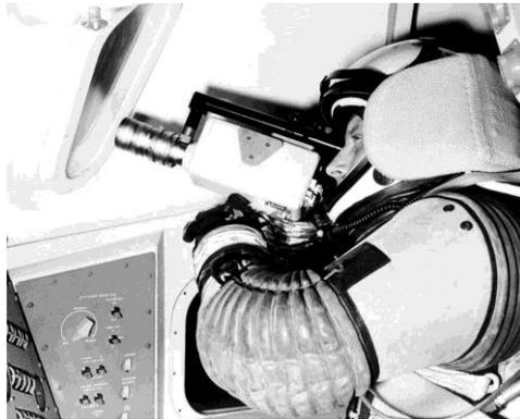
**Figure 22–10:** The RCA camera with its Angénieux 6x12.5 zoom during *Apollo 1* ground testing [2].
