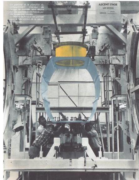
**Figure 22–32 (right):** LM Ascent Stage LTA-8 inner structure welding [Sciaky at Work Vol. 9 no. 2].
