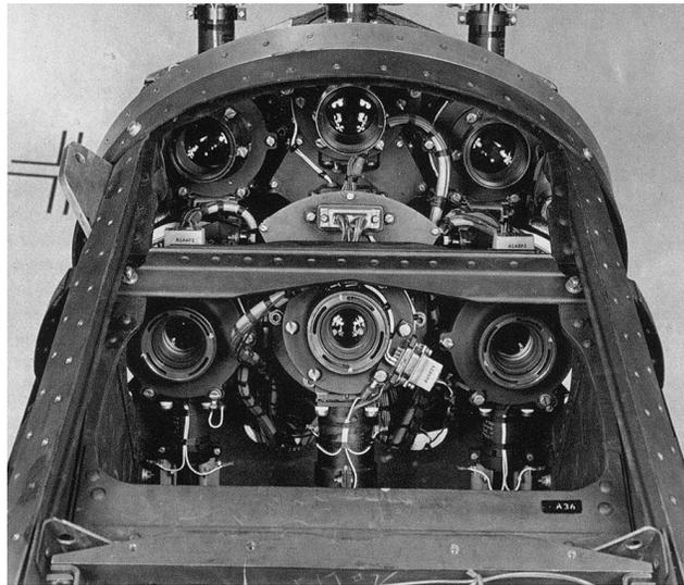
**Figure 22-3:** The three lower RCA cameras with Angénieux 25 mm lenses (FA in the middle). The upper cameras have B&L Super Baltar lenses [2].
