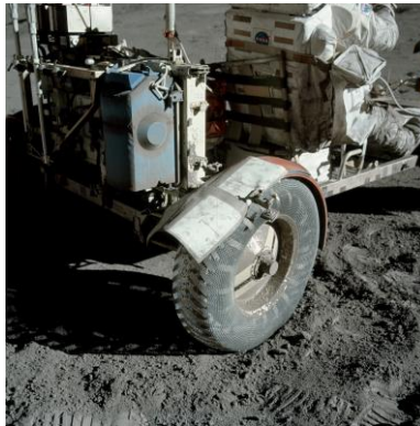
Figure 23–11 The broken rear fender of the LRV fixed by Gene Cernan (Apollo 17).
