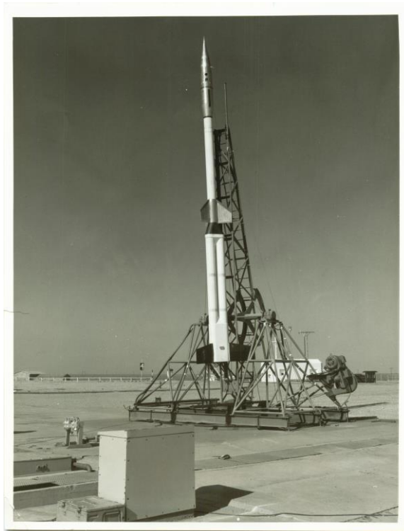
Figure 5-4: The Long Tom sounding rocket, a repurposed sighter rocket that replaced HARP to become Australia's first successful sounding rocket. Credit: DST Group.
