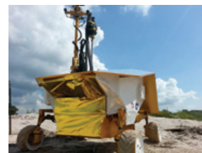
ABOVE NASA's Resource Prospector rover will carry out the first mining expedition on another world. The rover (now in development) will excavate volatiles such as hydrogen, oxygen, and water from the Moon.
