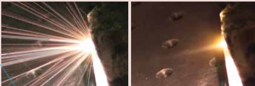
ABOVE Zapping olivine rock with a laser, this shows the ablation response of the olivine in the left photo with ejecta (pieces) coming out, and on the right with a mini “rocket plume.”
