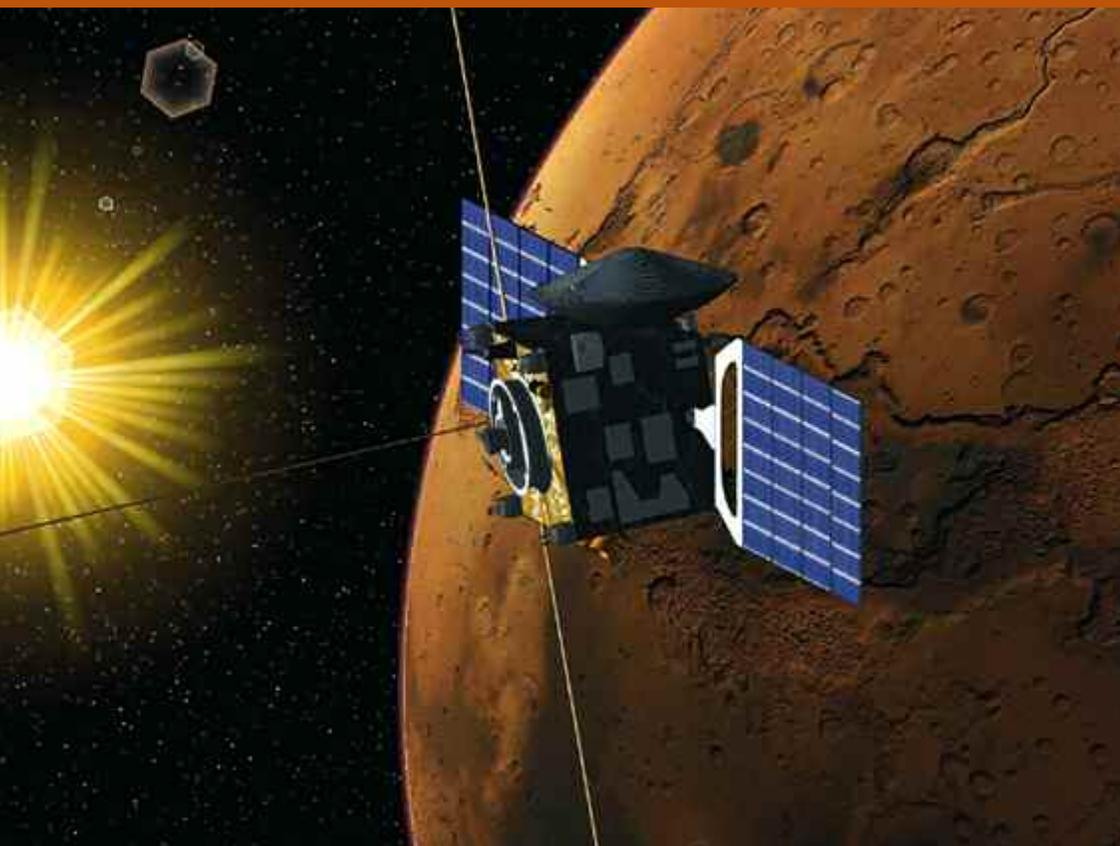
*As Mars Express enters eclipse around Mars, it flies in a survival-mode configuration nicknamed Sumo. In this artist's illustration, Mars Express is shown in a power-saving warm-up attitude, with its base pointed toward the Sun to catch the most heat.*
