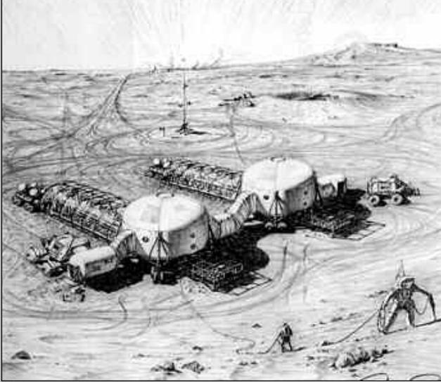
*redundant systems in case of emergency or equipment failures. Each HAB has an attached, inflatable greenhouse, airlocks, and rock sample racks accessible by robot arms, and a small airlock for hands-on examination. In a nearby crater, a small nuclear generator provides initial electrical energy.*
