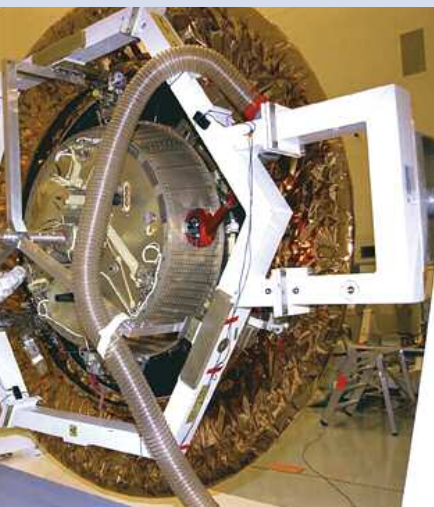
A worker inspects Huygens' heat shield after installation at Kennedy Space Center's Payload Hazardous Servicing Facility in July 1997.
