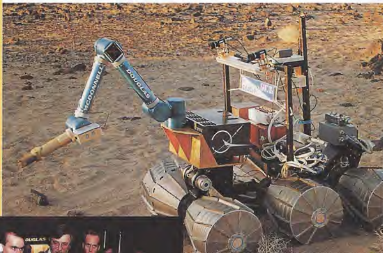
Above: The rover's familiar appearance changed for parts of these tests with the addition of a manipulator arm built by McDonnell Douglas Aerospace. Photograph: James D. Burke
