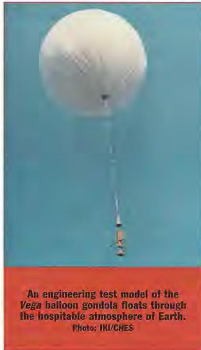
An engineering test model of the *Vega* balloon gondola floats through the hospitable atmosphere of Earth.
