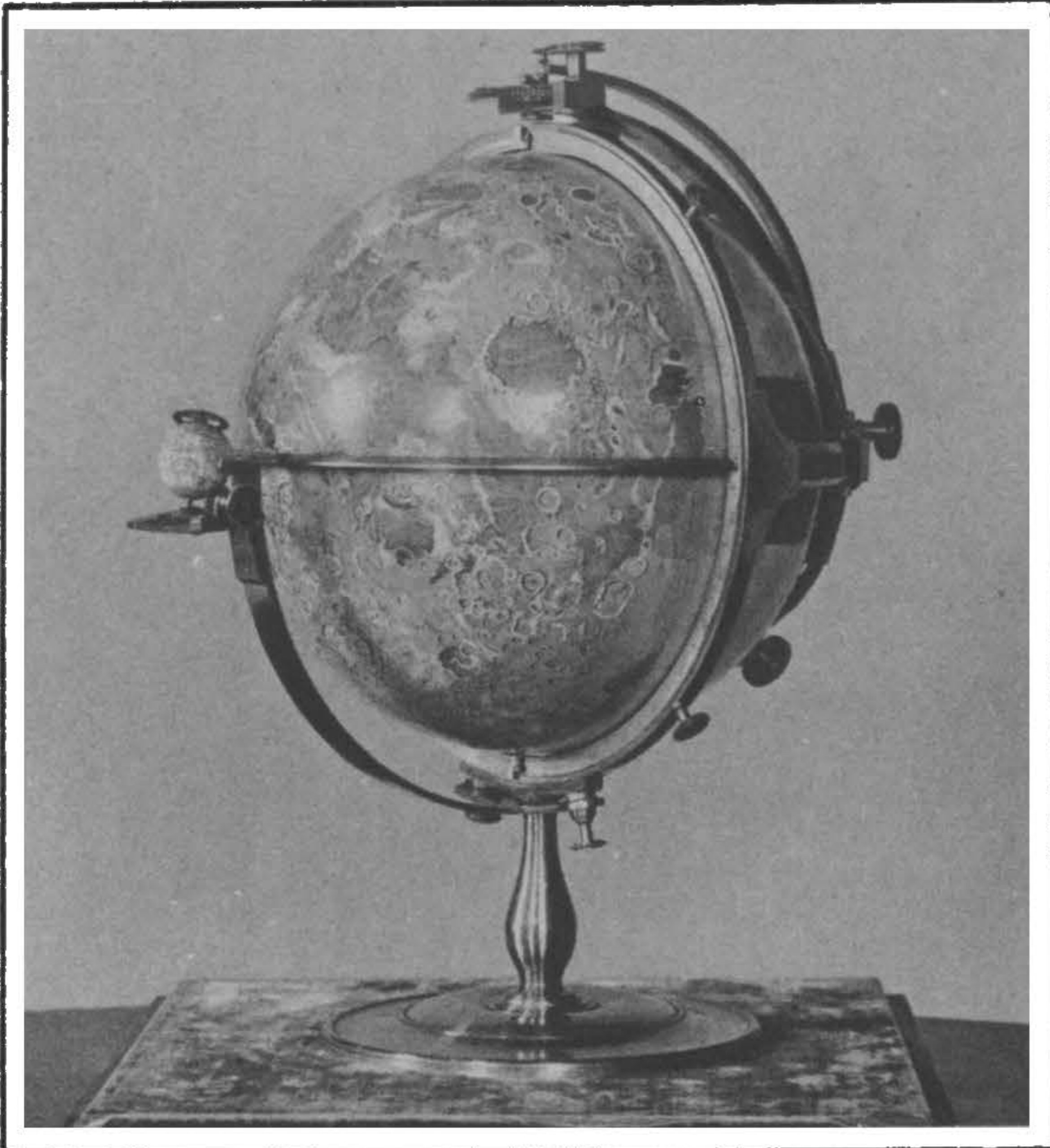
THE "SELENOGRAPHIA" INVENTED BY JOHN RUSSELL: A GLOBE SHOWING THE VISIBLE SURFACE OF THE MOON.
