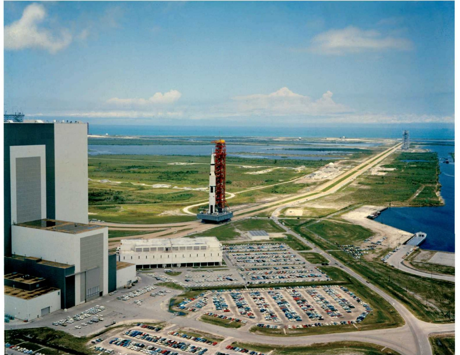
An aerial view of Cape Kennedy, May 20, 1969, shows the Saturn V rocket as it was transported down the 3.5-mile approach to Launch Complex 39A.
