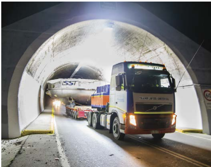
▲ TIGHT SQUEEZE After arriving at the port of Coquimbo in Chile in 2018, the telescope’s coating chamber was divided into two parts like an Oreo and transported to the summit of Cerro Pachón. Along the way, hanging signs, utility cables, and lights had to be removed to make room. Here, the chamber makes its way through the narrowest tunnel along the route. (Planners decided the telescope’s size with this tunnel in mind.)
