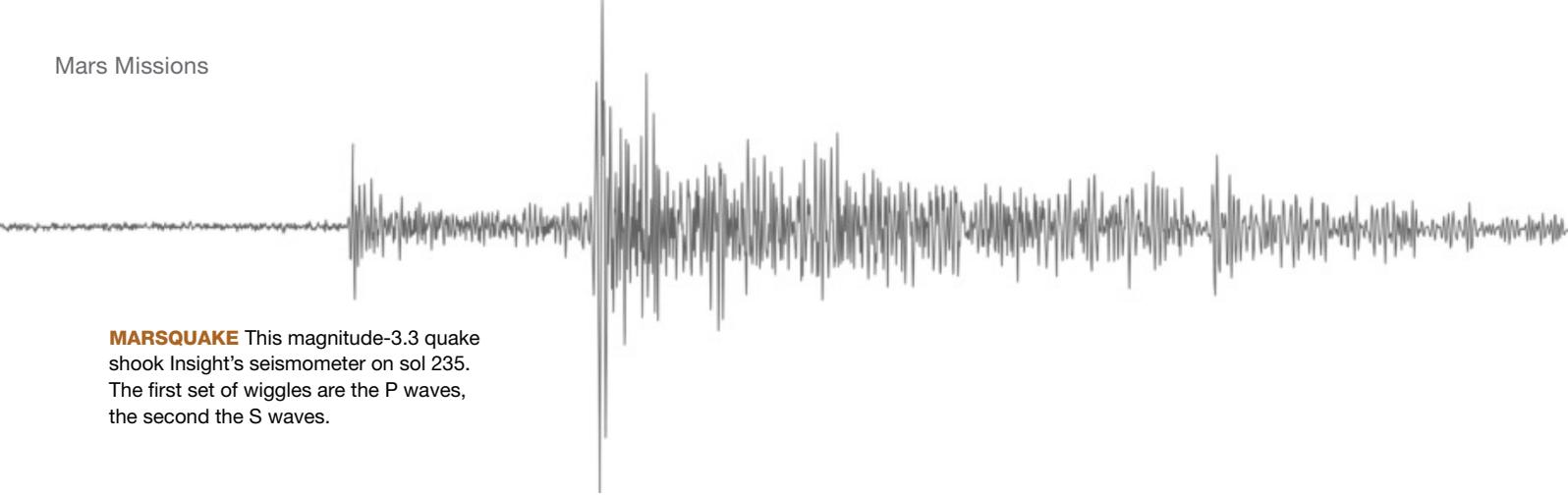
**MARSQUAKE** This magnitude-3.3 quake shook Insight's seismometer on sol 235. The first set of wiggles are the P waves, the second the S waves.
