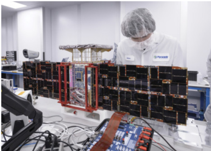
▲ CAPSTONE A team member installs solar panels on the CAPSTONE spacecraft. Despite multiple mishaps, the little satellite successfully reached the Moon in late 2022.
