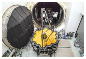
CHAMBER A Webb emerges from months of cryogenic vacuum testing in 2017.
