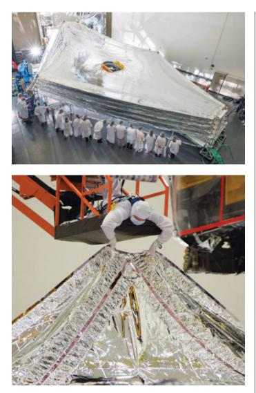
▲ **SUNSHIELD** *Top:* This photo from 2014 shows the first time engineers stacked and unfurled a full-size test sunshield. *Above:* A technician carefully folds the real sunshield in 2020, in preparation for stowing the telescope into its launch configuration.
