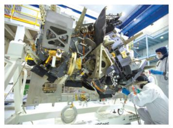
▲ **MEGASIZE INSTRUMENTS** Engineers prepare the Near-Infrared Spectrograph for acoustic tests.
