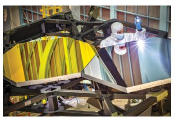
▲ **GO FOR GOLD** An optical engineer examines two test mirror segments, one coated in gold. The frame is a composite material designed to handle Webb's space environment.
