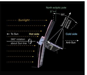
▲ **THE VIEW** Webb's mirror is perpendicular to its sunshield, and the spacecraft can tilt to point the telescope within a 50° arc while still keeping the mirror and instruments safely in shadow. It can also rotate full circle. Over time, Webb will see the entire sky as it orbits the Sun.
