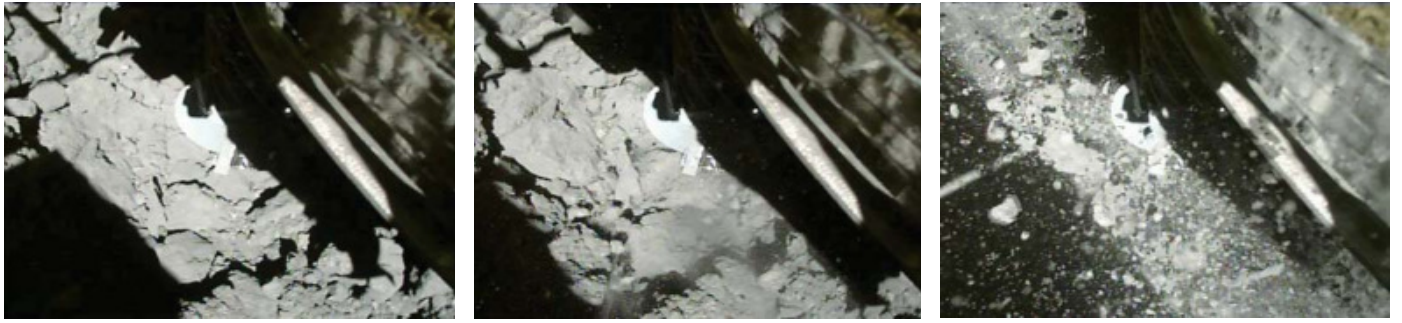
▲ TOUCHDOWN Hayabusa 2 executed its second touchdown on July 11, 2019, near Ryugu's equator. The images capture 4 seconds before, the moment of, and 4 seconds after touchdown.
