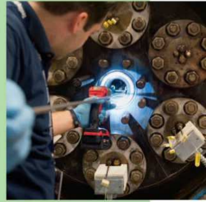
▲ TO HELL AND BACK NASA Glenn engineer Kyle Phillips removes samples from GEER after they were exposed to Venus surface conditions for 80 days.
