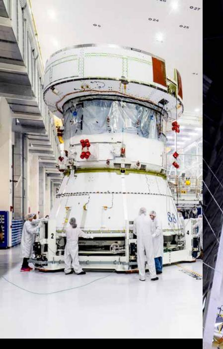
Also at the O&C, Orion's Artemis 1 service module moved across the air bearing floor to the lift station inside the assembly bay, where it underwent installation and fastening to prepare it for its own acoustics testing. Just as the crew module underwent testing, the service module was surrounded with speakers and exposed to the acoustic levels that it will experience on its journey into deep space.
