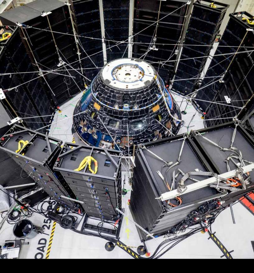
In the Operations and Checkout Building (O&C) at NASA's Kennedy, Orion's Artemis 1 crew module recently underwent Direct Field Acoustics Testing where it was exposed to maximum acoustics levels that the vehicle will experience
