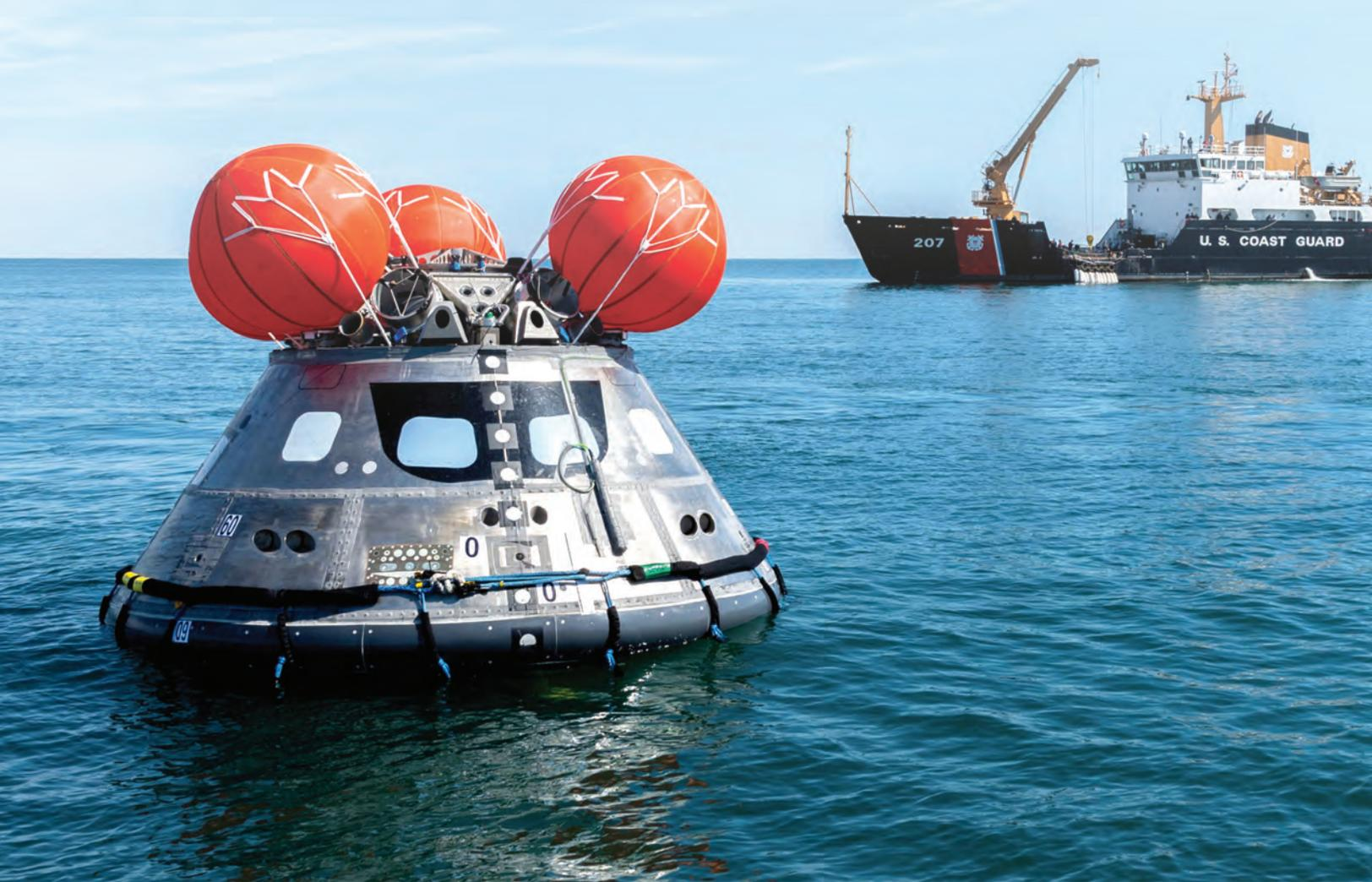
Engineers completed two key tests the week of March 18 to help ensure NASA's Orion spacecraft is ready from liftoff to splashdown for missions to the Moon. Teams successfully tested one of the motors on Orion's Launch Abort System responsible for taking the crew to safety in an emergency during launch, and completed testing at sea for the qualification of the system used to upright Orion after it lands in the ocean.
