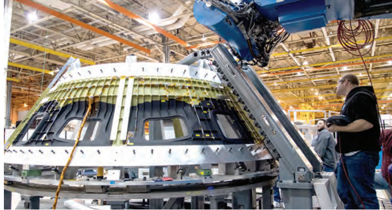
Lockheed Martin engineers at NASA's Michoud Assembly Facility in New Orleans, weld the cone section for the Orion spacecraft which will carry humans beyond the Moon on Exploration Mission-2.
