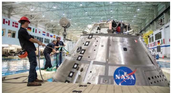
The team is conducting development tests for the Orion Crew Module Uprighting System (CMUS) using the PORT test article, a full-scale mockup of the Orion crew module, in the Neutral Buoyancy Laboratory at NASA's Johnson Space Center in Houston.
