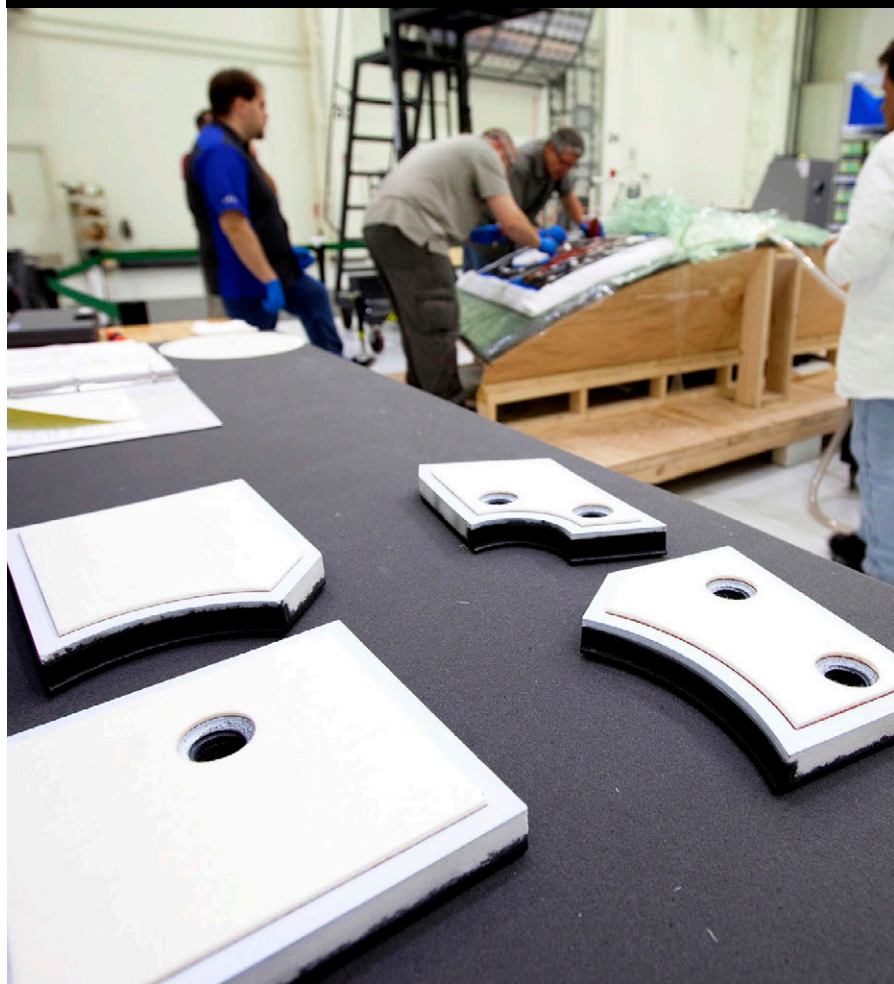
Technicians prepare to bond thermal protection system tiles on the Orion crew module for the agency's Exploration Mission-1 flight with the Space Launch System (SLS) rocket. Orion requires about 1,300 tiles. Many of the Orion tiles are standard, except for those which fit around windows, thrusters or antennae. Along with the spacecraft's heatshield, the tiles will protect Orion from the 5,000 degree Fahrenheit heat of re-entry.
