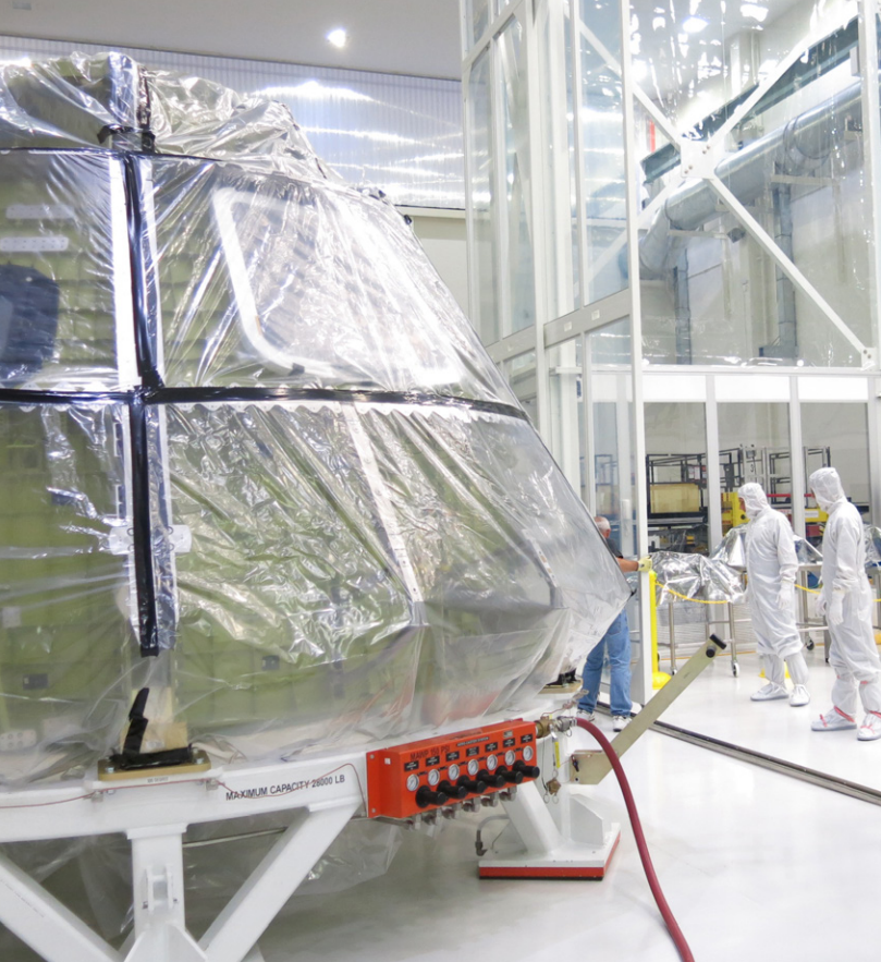
The Orion crew module for Exploration Mission-1 is transferred into the clean room inside the Neil Armstrong Operations and Checkout Building at Kennedy Space Center for installation of the spacecraft's critical systems, including propellant lines.
