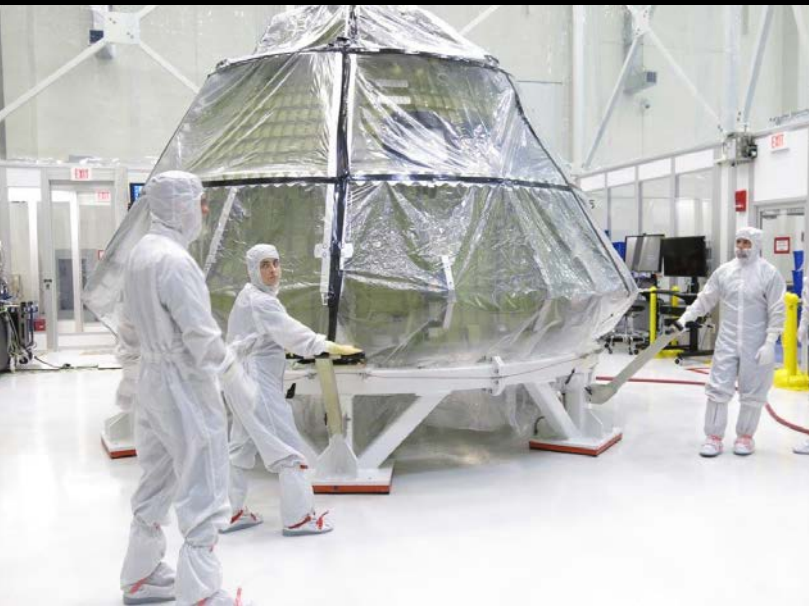
The Orion crew module for Exploration Mission-1 is transferred into the clean room inside the Neil Armstrong Operations and Checkout Building at Kennedy Space Center for installation of the spacecraft's critical systems, including propellant lines.
