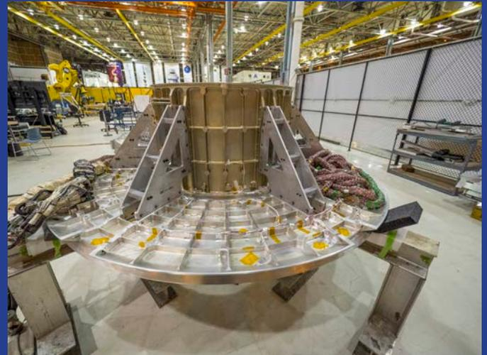
Pieces of the Exploration Mission-1 Orion spacecraft being prepped for welding at NASA’s Michoud Assembly Facility.
