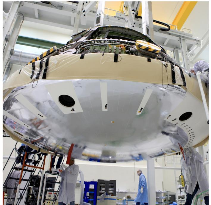
Orion's reentry into the atmosphere, preventing heat from being transferred to the rest of the crew module.
