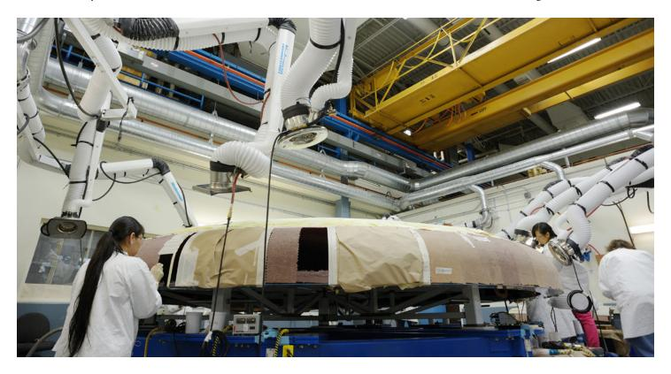
Progress continues toward completion of the Orion Exploration Flight Test-1 (EFT-1) heat shield at Textron Defense Systems in Wilmington, Mass.
