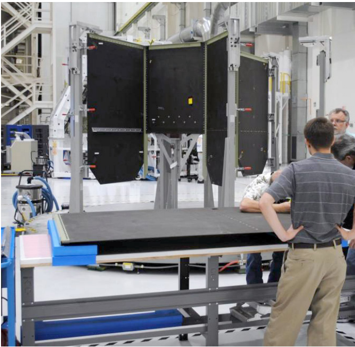
All six EFT-1 Service Module shear panels were fastened and ground test instrumentation wires and sensors were mounted on the shear web assembly tool in Kennedy Space Center's Operations & Checkout Building.
