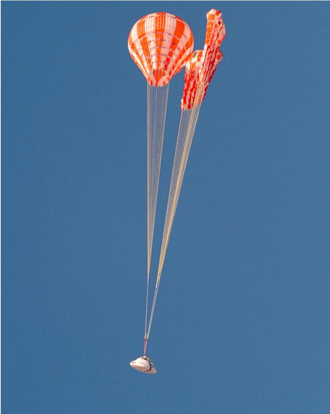
The parachute team completed another successful airdrop test on July 18 at the U.S. Army's Yuma Proving Grounds in Arizona in preparation for the vehicle's orbital flight test in 2014. The test was the second to use the Parachute Test Vehicle (PTV) to represent the size and shape of the Orion Crew Module including a representative spacecraft parachute compartment.
