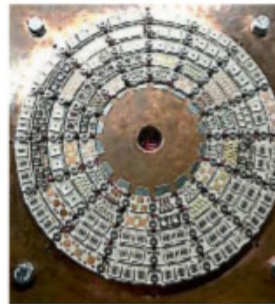
The LED simulator that was used to mimic a red dwarf star’s light in experiments on Earth
