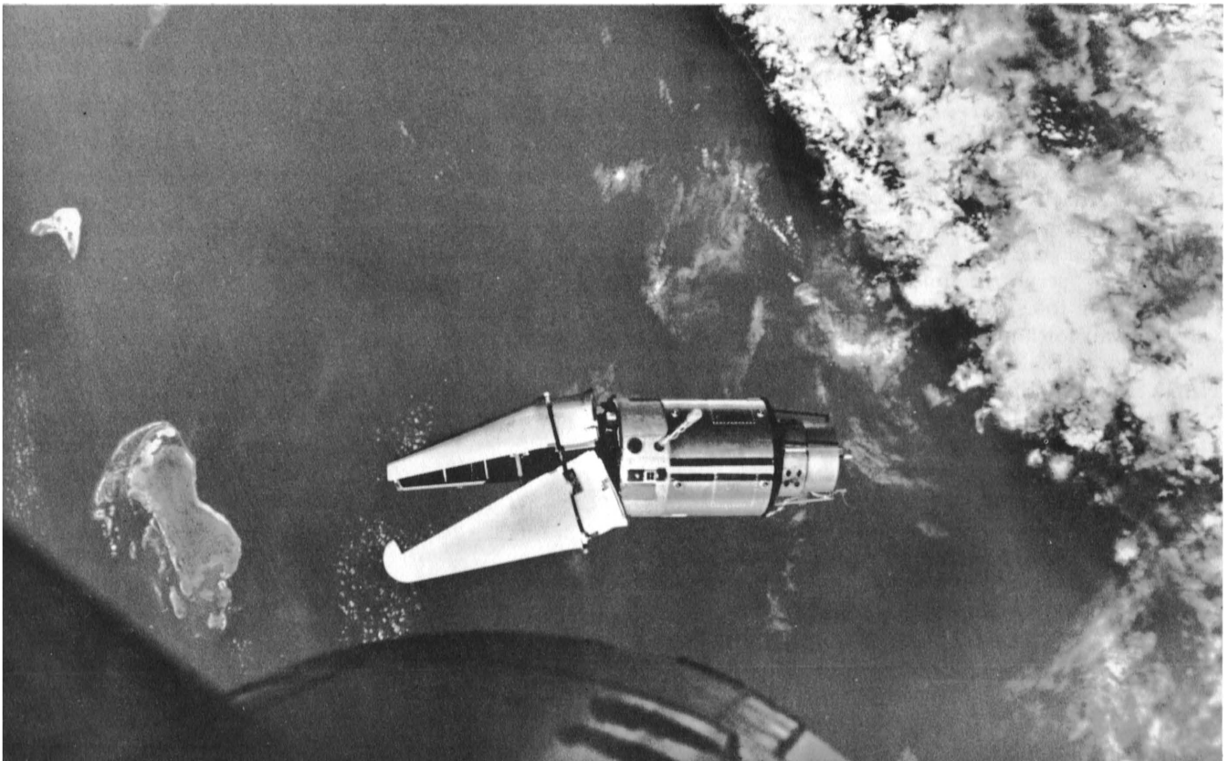
THE AUGMENTED TARGET DOCKING ADAPTER as seen by the Gemini IX spacecraft after the rendezvous in space. Command pilot Tom Stafford referred to the ATDA and its still attached shroud as an "angry alligator."
